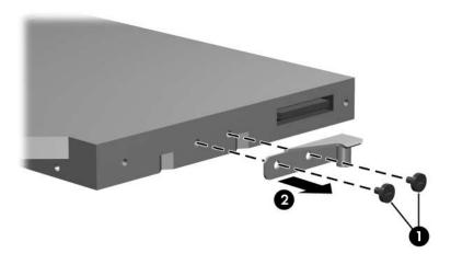
Removing the Optical Drive Bracket
